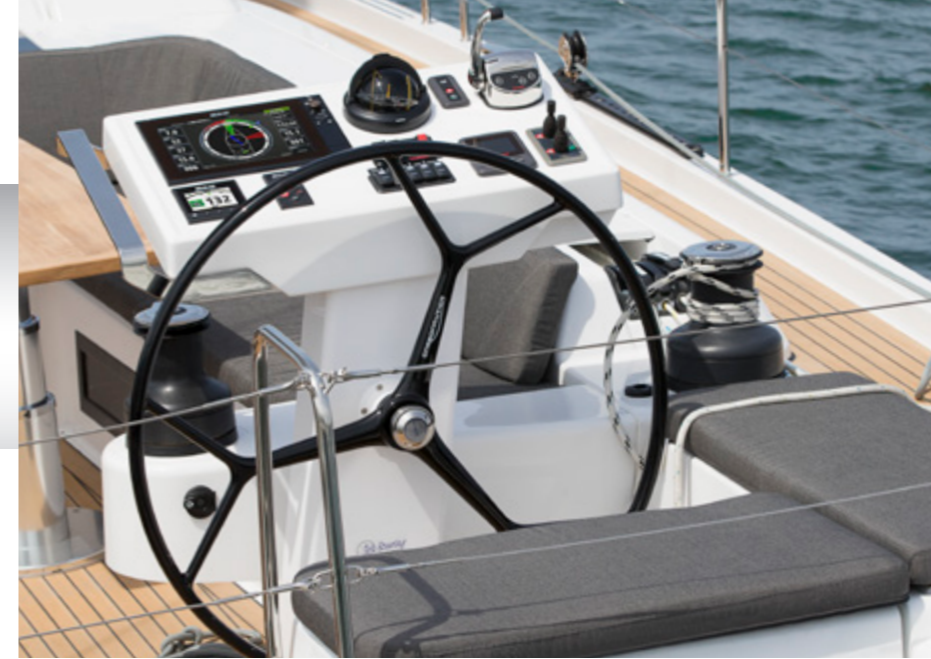
2 instrument pods | B&G Autopilot with Triton 2 control unit and precision 9 compass GoFree wireless link | VHF preparation with antenna and splitter for FM and AIS
